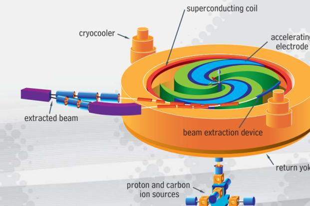
Engineer view of the C400 superconducting cyclotron
